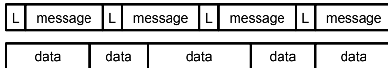
Figure 10.6: DNS messages over TCP streams are not necessarily aligned to TCP segments.
